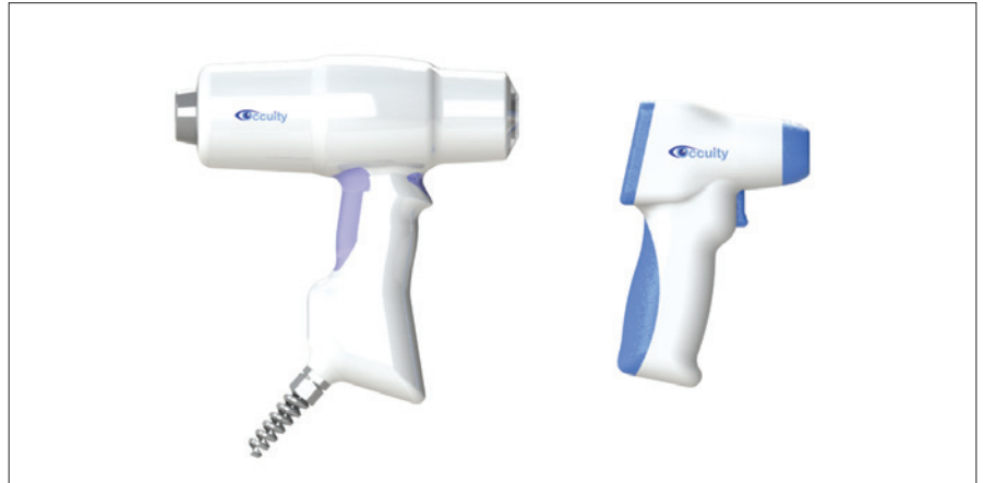
The proof of concept device, which connected to a computer rather than having an inbuilt display. Right: Garage ‘prototype’, fully integrated with a camera and touch screen display on the back, with all processing embedded in the electronics © Occuity
