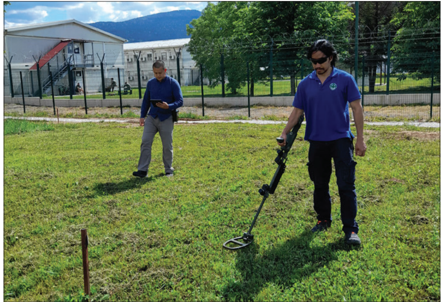
MiFi Maps' roving tracking device being tested during a field trial in Sarajevo, in this case attached to a metal detector © MiFi Maps
