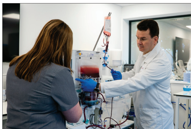
Usability is a key feature of any biomedical device, embodied in the design of the OrganOx metra so that it self-fills from the bottom up while effortlessly expelling air at the top of the device
