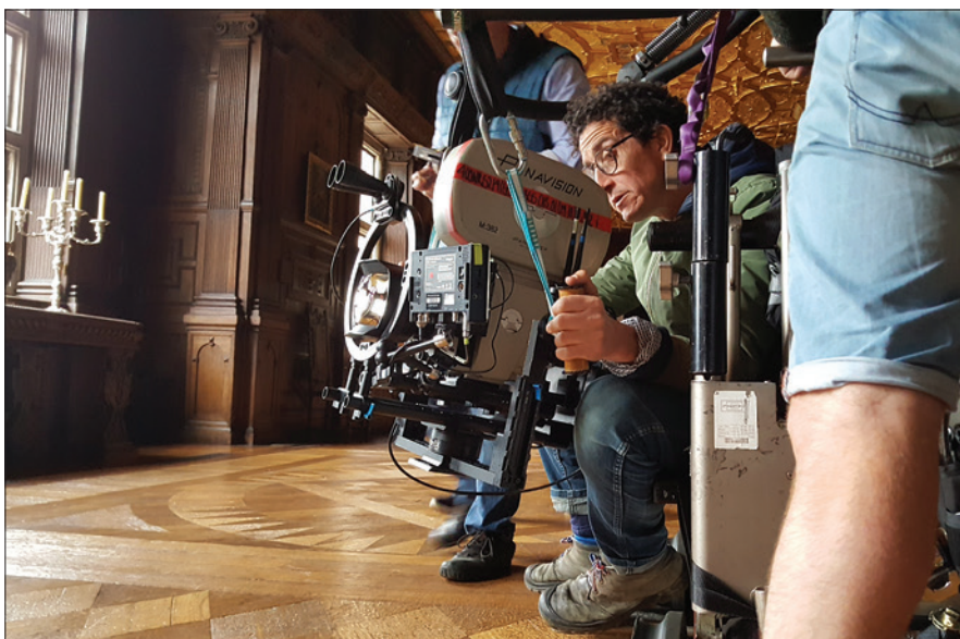
Robbie Ryan BSC ISC shooting The Favourite with the Helix and exoskeleton arms customised to attach to a dolly. This was a first time such technologies were used and combined in this way, with a Panavision XL2 35mm film camera attached to the exoskeleton and to the dolly where the operator has freedom of movement in a unique way © Pixeled Pictures
