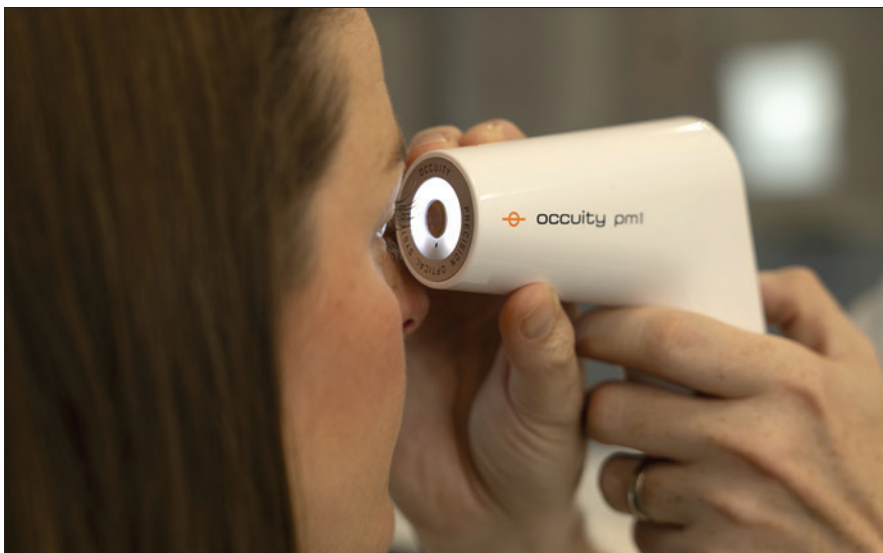
Occuity's handheld PM1 device supports glaucoma detection, and takes just a few seconds to scan the eye. The company is also developing oculosics devices that will share many of its design features, but will instead allow clinicians to test for chronic health conditions such as diabetes and Alzheimer's © Occuity
