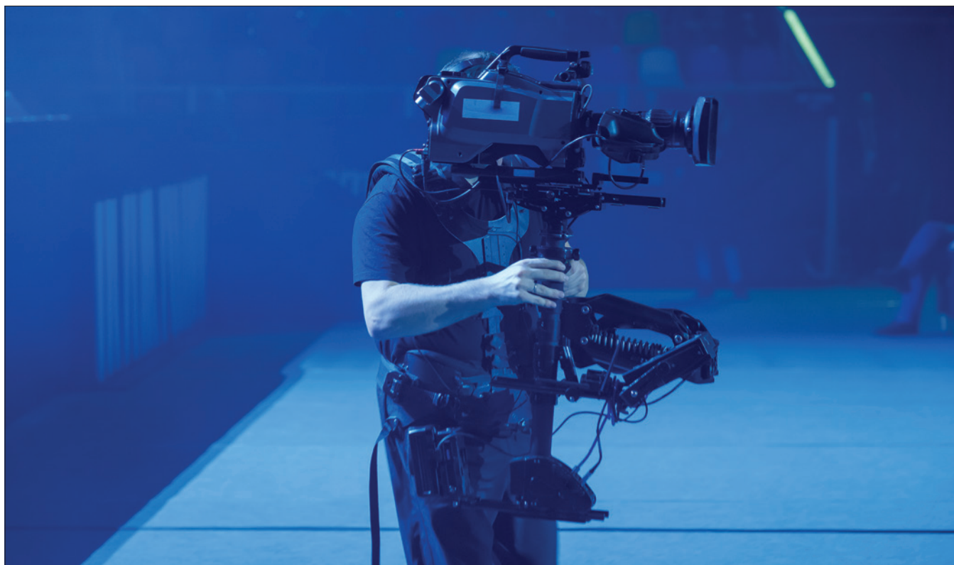
The Steadicam, invented by camera operator Garrett Brown in the 1970s, allowed effortless continuity in cinema for the first time. It both isolates the operator's movements from the camera and distributes the camera's weight through the operator's vest © Shutterstock
