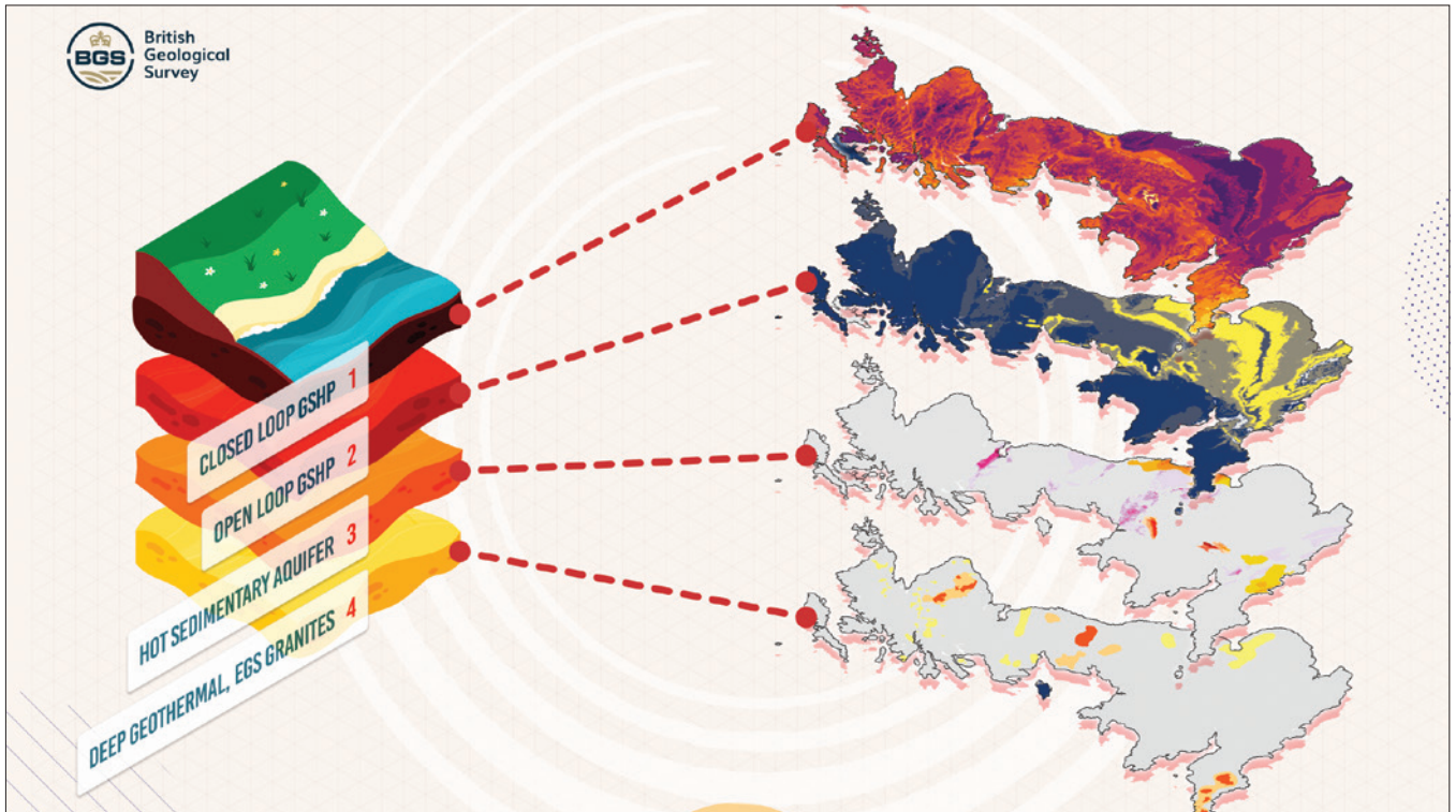
Overview of geothermal energy potential for four geothermal technologies in the UK: Closed loop ground source heat pumps (GSHP), open loop ground source heat pumps, hot sedimentary aquifer and deep geothermal, EGS granites. (Contains OS data © Crown Copyright and database right 2025, data © Department for Energy Security and Net Zero, 2025, data BGS © UKRI 2025.)
