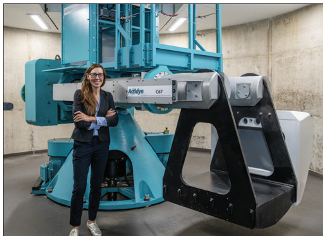
Gourvenec with the 6-metre diameter geotechnical beam centrifuge at the National Infrastructure Laboratory, which allows geotechnical engineers to scale up stresses to scaled-down models and test a design life of loading in a highly controlled, instrumented environment
