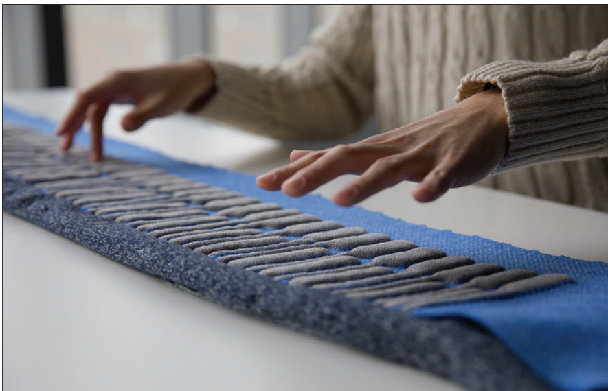
Irmandy Wicaksono's knitted keyboard can be controlled by touch, pressure, stretch, and even just proximity: a musician can play by hovering their hands over it, similarly to a theremin © Irmandy Wicaksono
