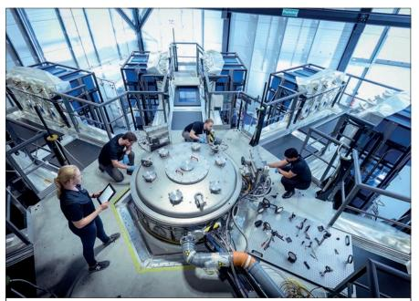
'Machine 3', built in 18 months at a cost of £3.6 million, stores electrical energy in banks of capacitors. It uses electromagnetic forces to launch projectiles at the hypervelocity speed needed to test fusion targets. The projectiles hits the amplifier at 20 km/second. The company describes this as "one of the largest pulsed power facilities in the world and the largest in Europe". It is also the only one built specifically for fusion research © First Light Fusion
