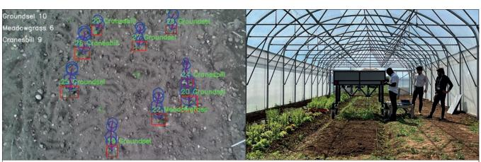
Computer vision software identifies different species of weed (left) and the autonomous spot application of herbicide robot in action (right) © Warwick Agri-Tech at WMG, University of Warwick
