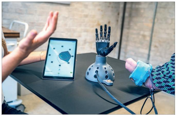
Calibration of Ottobock's myoelectric prosthetic hand takes place when an individual first receives the devices © Ottobock
