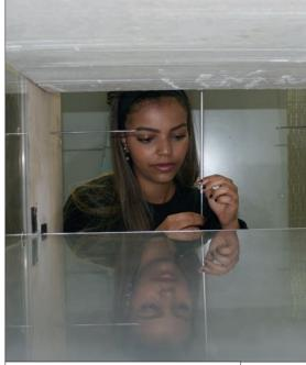
Abigail sets up an experiment by placing a total pressure pitot into its holder in her experimental rig
