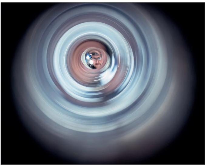
It takes 3 kilograms of gunpowder to set off First Light Fusion's two-stage big friendly gun to blast a projectile at a target that contains fusion fuel. The company first achieved fusion in 2021 © First Light Fusion
