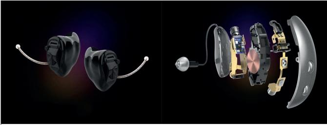
Starkey has incorporated its Genesis AI hardware into its invisible hearing aids (which are fitted in the ear canal and cannot be seen on the outside of the ear), as well as larger models of its hearing aids © Starkey
