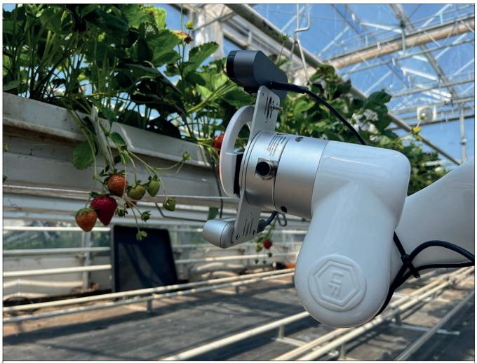
Robots are increasingly being used for autonomous monitoring and inspection. Here, the robot is checking the ripeness of strawberries but the same set up can monitor for other things such as pest and diseases © Warwick Agri-Tech at WMG, University of Warwick
