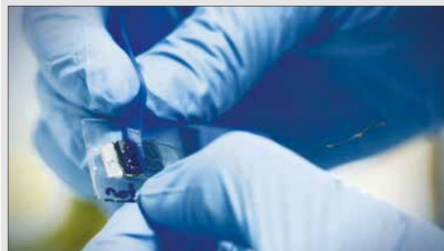
A variety of methods exist for producing graphene on a mass scale, but Scotch Tape remains a favourite in labs across the world © University of Manchester
