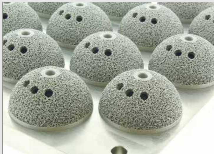
Recent advances in AM include the development of load-bearing lattice structures for orthopaedic implants. By incorporating a lattice, implants can provide a scaffold structure for new bone tissue to grow into, with the spacing and strut thickness of the lattice optimised to match the stiffness of surrounding bone. The lattice, with its ‘pseudo-random’ internal structure, would be near impossible to manufacture in any other way than AM © Renishaw
