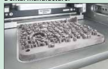
The build file is then used to manufacture parts. There could be 200 to 300 parts on one plate.
