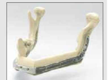
The new jaw, with the two sections of bone from the fibula connected to the remaining jaw either side by an AM-produced titanium plate © Renishaw
