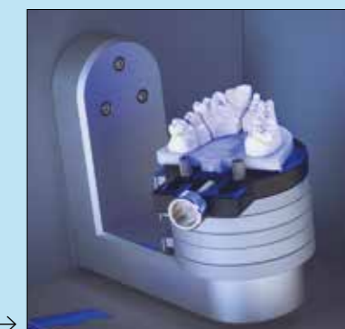
A lab scanner digitises the model, often using structured light scanning.
