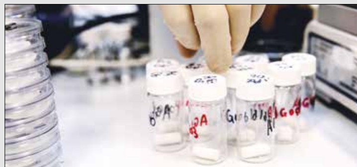
Aerograft is a bioactive aerogel silicate-based material with calcium and phosphate ions. The material is used to improve the stability of implants in several dental and orthopaedic procedures
