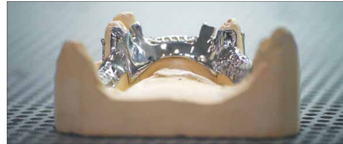
Additive manufacturing can capture the complexity of removable partial dentures © Renishaw
