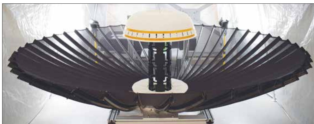
Oxford Space Systems' deployable structures, such as this wrapped-rib antenna, use novel design techniques based on origami so that they can be folded and stowed more efficiently © Oxford Space Systems
