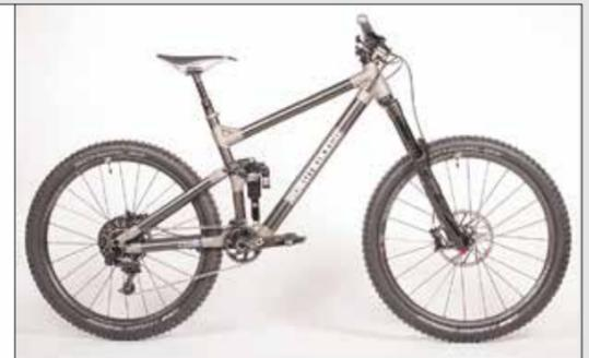
The titanium lugs for Robot Bike Co.'s bespoke MTB bike frame were produced using Renishaw's selective laser melting process, an additive manufacturing technology that can build components directly from computer-aided design geometry using fine metal powders © Renishaw/Robot Bike Co.
