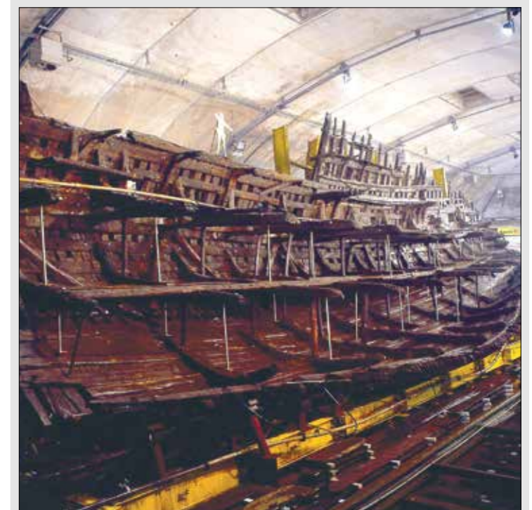
Sprays cover the Mary Rose hull with water in 1991. The hull is still on the same yellow cradle that lifted it out of the sea in 1982. It sits on the barge deck, which was cut away when it arrived at the dry dock, and rests on brick piles at a slight angle so that water and PEG solutions could drain away © Mary Rose Trust
