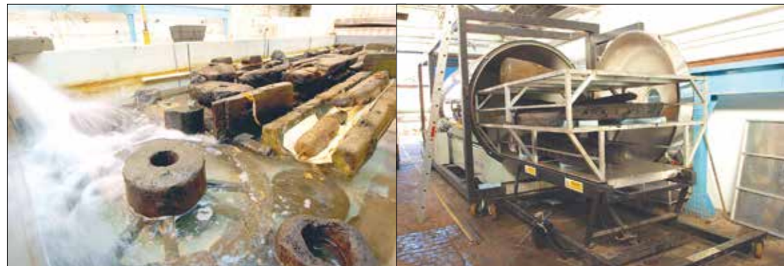
The Mary Rose team soaks the wooden artefacts in PEG for a few years and then, because they still have water in them, freeze-dry them. At six metres long, the Mary Rose freeze dryer (right) is the largest in the country. The chamber freezes the items and any remaining water turns to ice. A vacuum then applies pressure that causes the ice to sublimate and turn straight from solid to gas. Because the water comes out very quickly, it means that the dimensional changes are minimal and the process is relatively quick. The gun carriages, for example, only took three months © Mary Rose Trust
