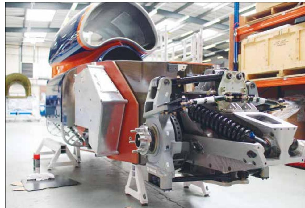
The Bloodhound's steering suspension joint is split and truncated, and the two parts move independently of each other. This gives the best suspension stiffness and prevents the wheel from flexing off line, which can cause instability © Stefan Marjoram
