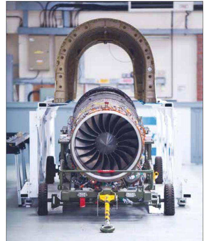
The Bloodhound was fitted with a jet engine designed for use in military fighter aircraft. This proved to be something of a challenge and resulted in changes to the shape of the car © Stefan Marjoram
