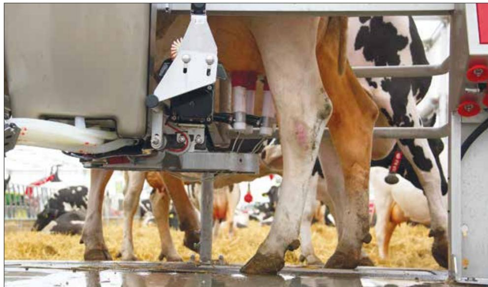
**A liquid flow sensor in the system that is electrochemically activated by milk can tell whether the cup is attached incorrectly and when the milk production has ceased, automatically allowing the suction cups to be removed. Inbuilt instrumentation can also run checks on the milk's quality and quantity** © Royal Association of British Dairy Farmers
