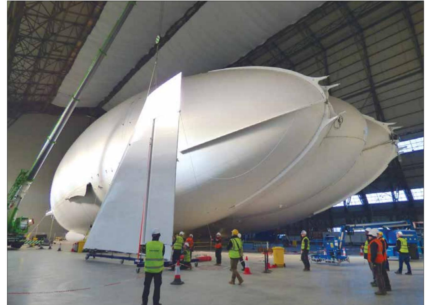
From the back, the Airlander resembles three sausages that have been squashed together, an arrangement that creates an aerodynamic shape, which is assisted by two top fins and two lower fins – one of which can be seen before it was attached to the hull © Hybrid Air Vehicles
