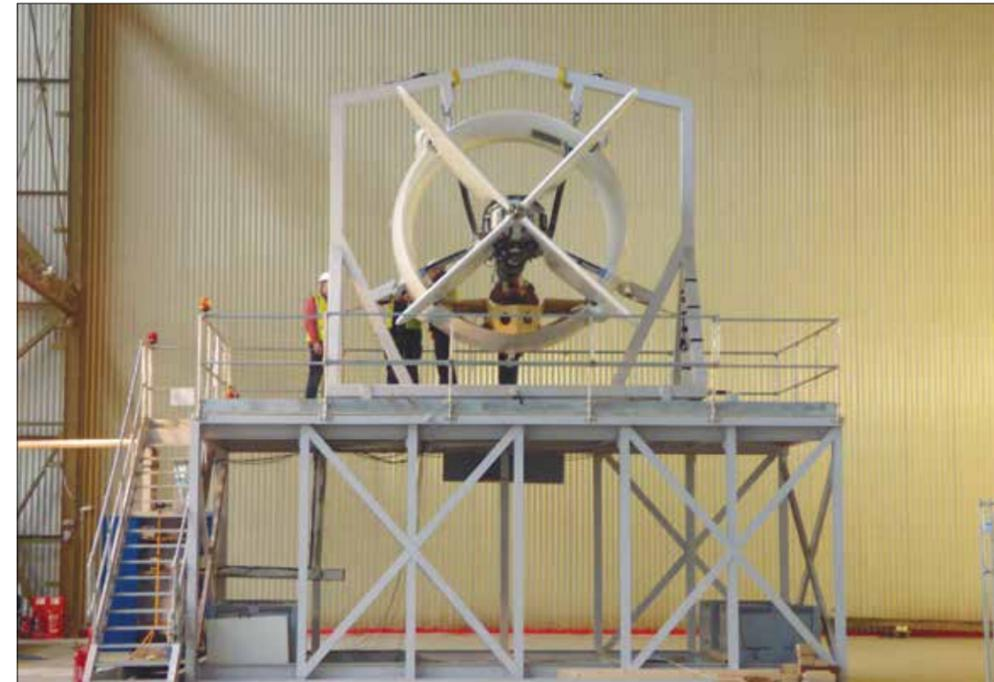
Four 325 horsepower turbocharged engines with variable pitch propellers power the Airlander. They are lighter than engines that were used for previous generations of airships and the absence of a rigid interior framework means that they need to be attached directly to the fabric structure of the craft © Hybrid Air Vehicles
