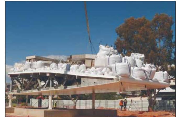
The prototype section of the canopy with its twin ferrocement shells and steel bracing being load tested in Athens. When the structure safely survived its anticipated failure loading, the team added concrete blocks to see when and how it would collapse, but they did not induce failure © Expedition Engineering
